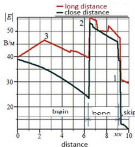
Figure 16 – Image of the field strength on the first and second floor of the head model (enlarged scale on the first floor of the head closest to the phone case)
